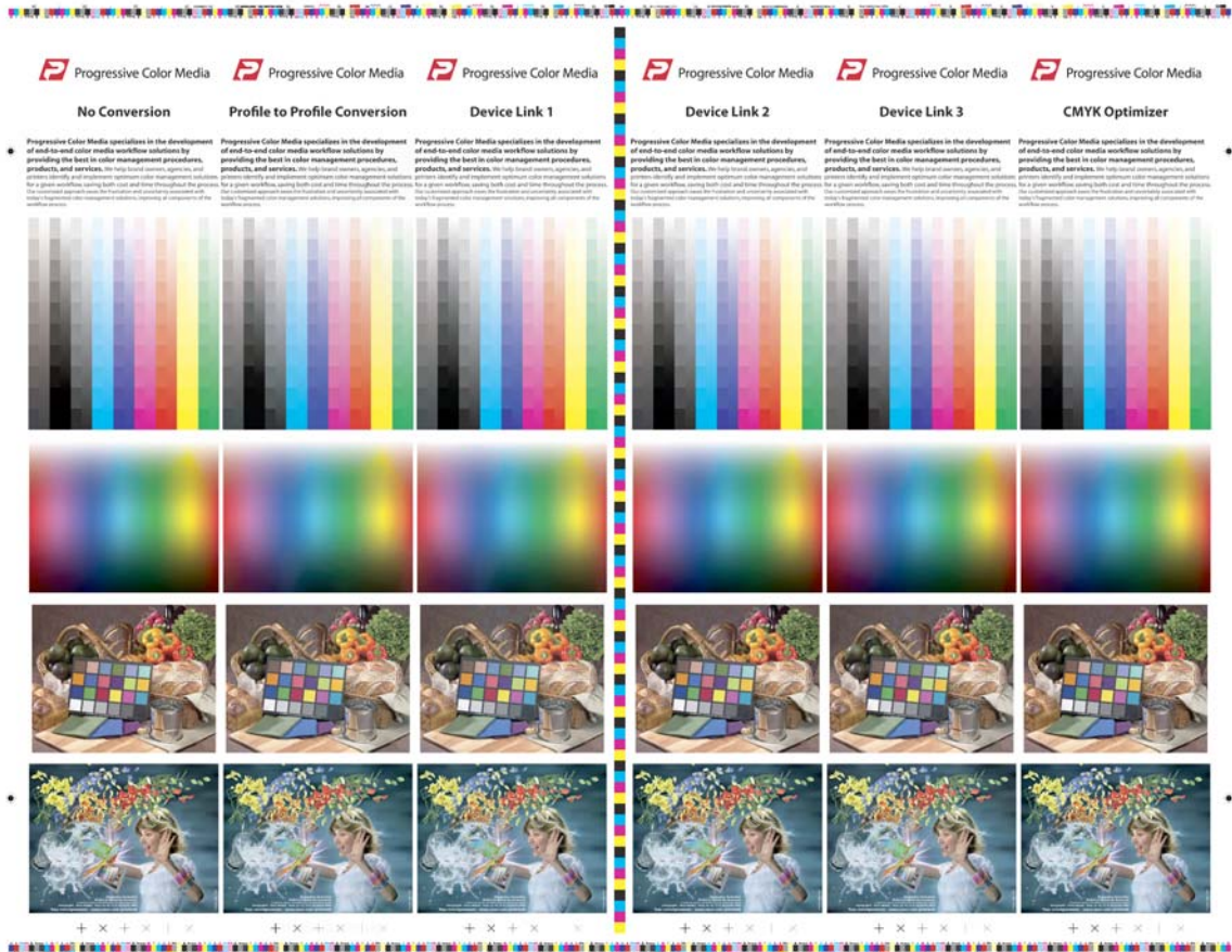
Figure 5: The test form used in phase 2 of the device link profile evaluation
